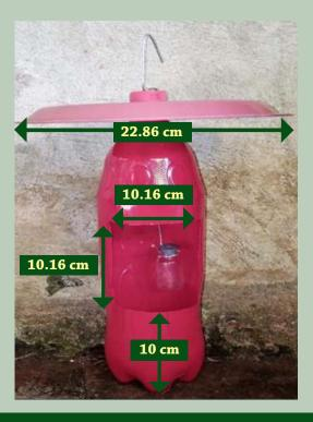
Figure 2. Modified lure trap
