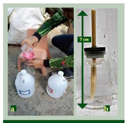
*Figure 1*. a) Preparation of methanol-ethanol ratio; b) Measurement of the bamboo stick in the vial
