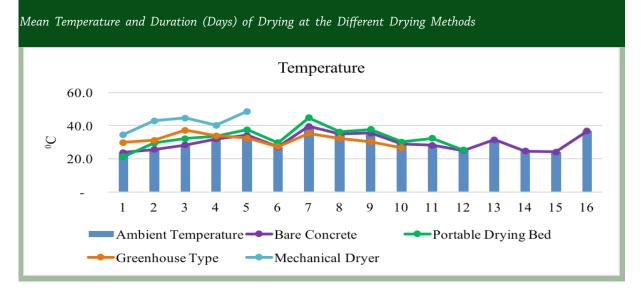
interval (9 AM, 12 NN, and 3 PM) using a digital thermohygrometer (Testo 608-H1) (Figure 2).
